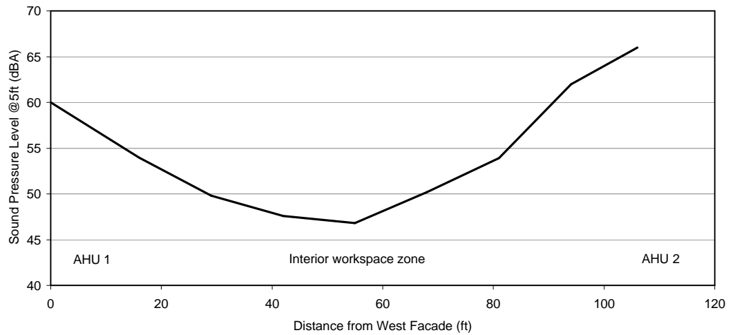
Figure 4.8 Ambient sound level readings
