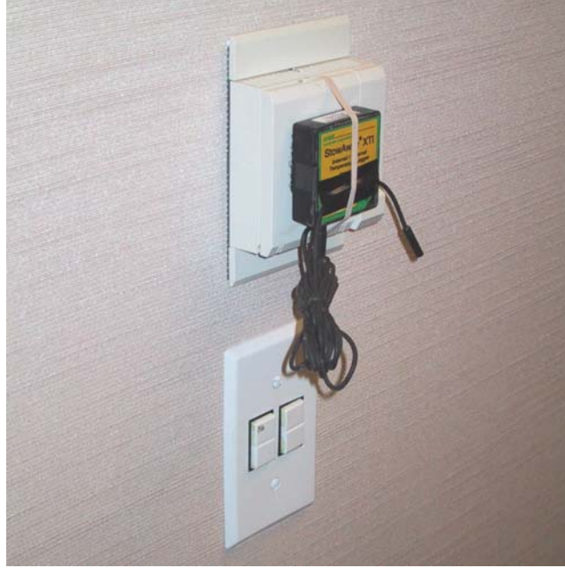
Figure 3: Example of logger and thermostat pairs used to evaluate time constant.
